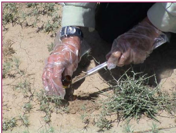
a. taking a soil sample from over a mine
