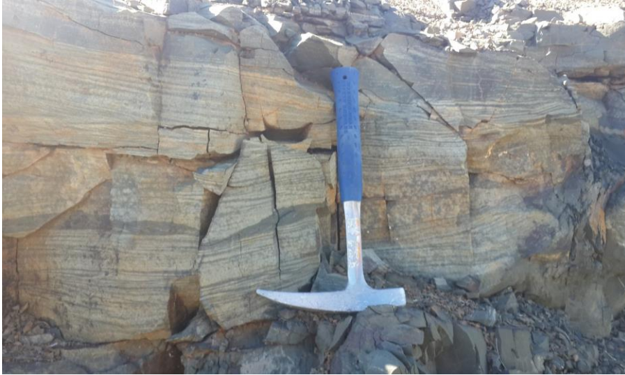
Figure 6.11: Horizontal and faint cross lamination in the sandstone of SFt facies.
