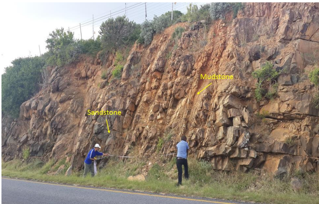
Figure 3.21: Photograph showing dark grey greywackes alternating with mudstones in the lower part of the Ripon Formation along the National road N2 between Grahamstown and Peddie.
