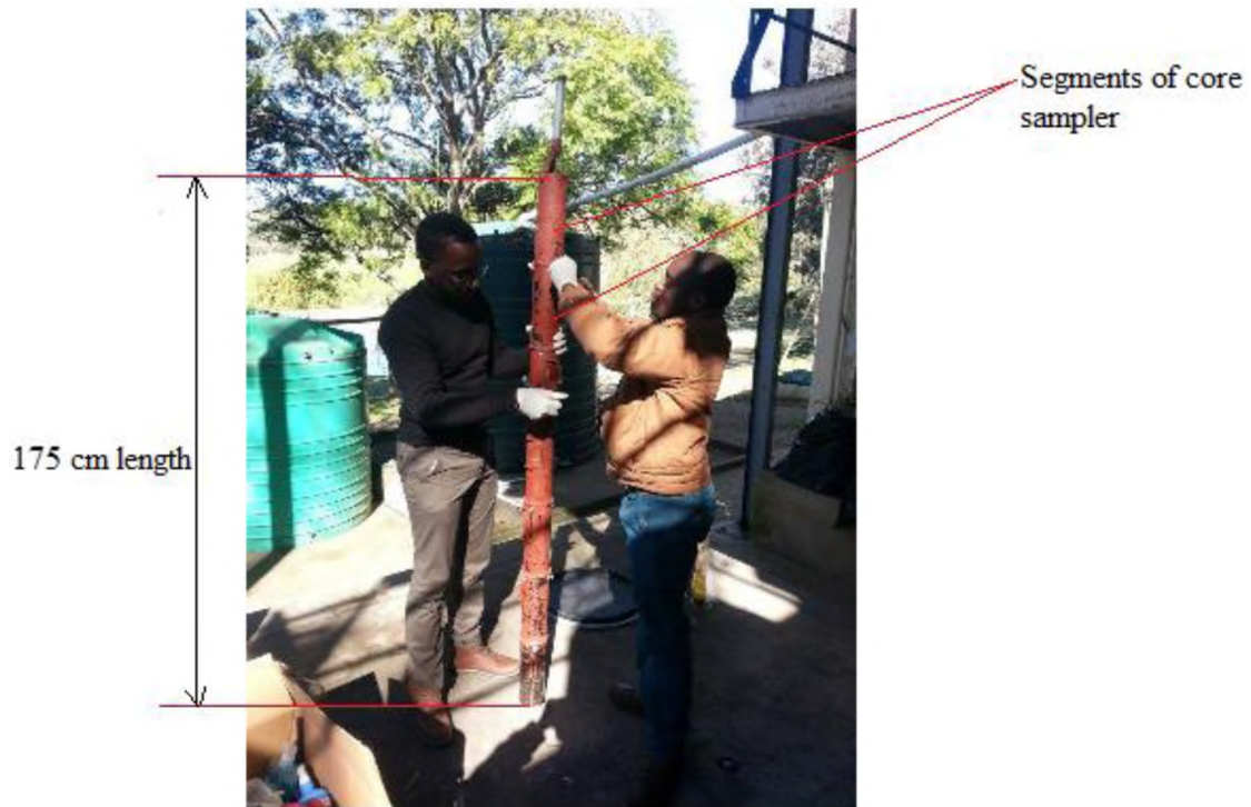
Figure 2.8: Showing core sampler used to sample pit latrines
