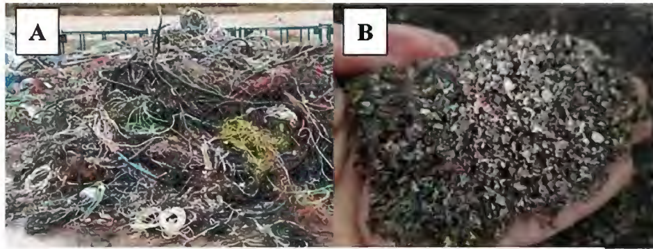
Fig. 1. (A) The cables awaiting recycling in the recycling plant. (B) Plastic waste product obtained after recycling. Source: Lyrsa Álava (Spain).
