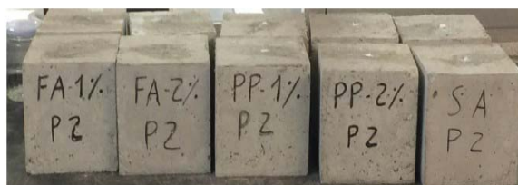
Fig. 1: Cubic specimens with additions of 1% and 2% by weight of FA and PP cement and without addition.
