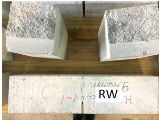
Fig. 5. Specimen with rockwool fibres after fracture parameter test
