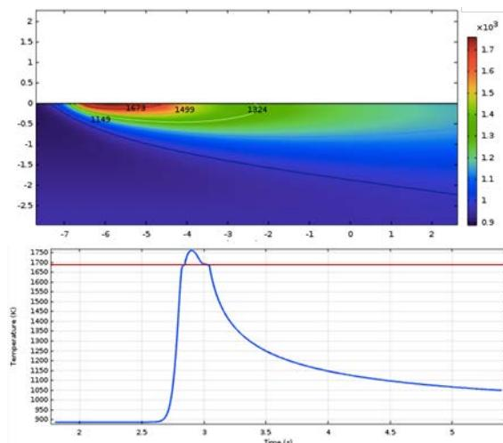
Fig 3: Temperature in the sample (top) and at a point versus time (bottom) obtained from the FEM model for a maximum optical intensity of 2700 W/cm<sup>2</sup> and a process velocity of 8.3 mm/s
