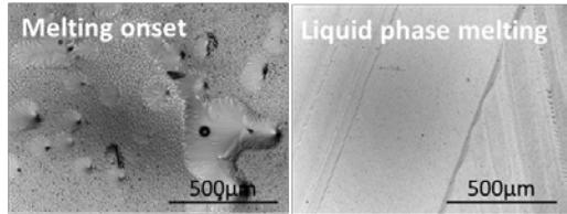
Fig 2: Onset of the silicon melting (left) and crystallized samples (right) obtained for different process parameters.
