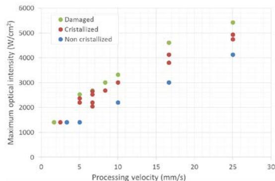
Fig 1: Parameter window for the silicon laser crystallization process.
