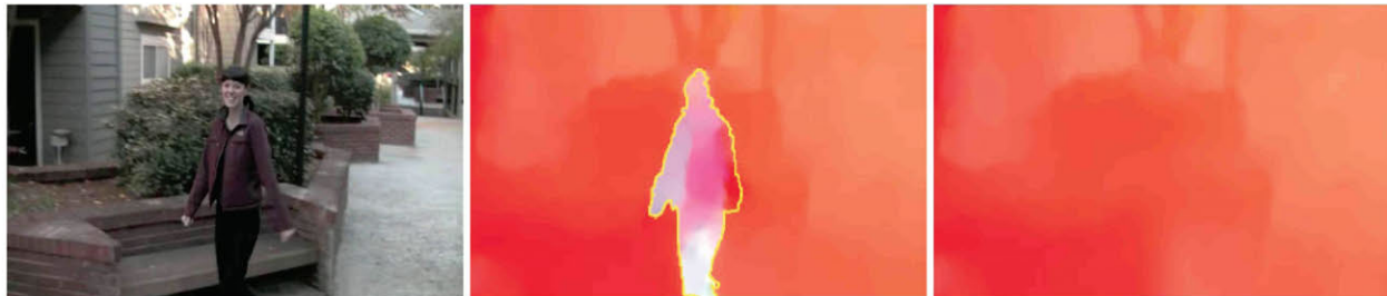
Figure 4. Outlier filtering with optical flow refinement. Notice the alignment between the motion vectors and the boundary in (b).
