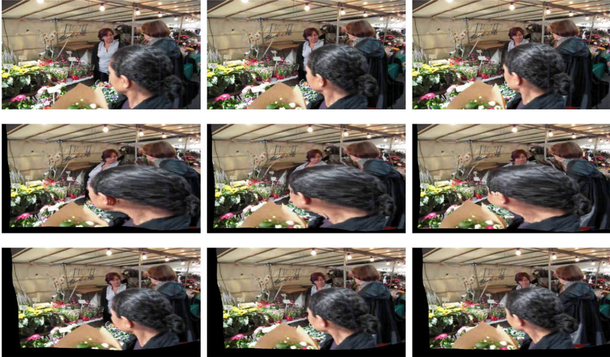
Figure 5. Typical failure case for trajectory based methods. Our system manages to stabilize this heavily occluded scene. The rows from top to bottom correspond to the original, stabilized without filtering and successfully stabilized cases. Notice the heavy distortions in the second row.
