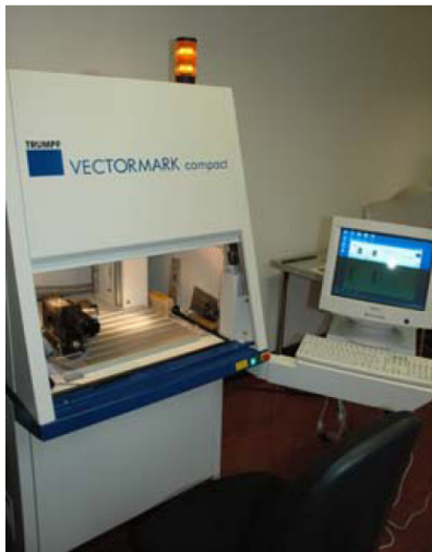
Figure 3. Micromarking system with Laser Trumpf VectorMark VWS 800
