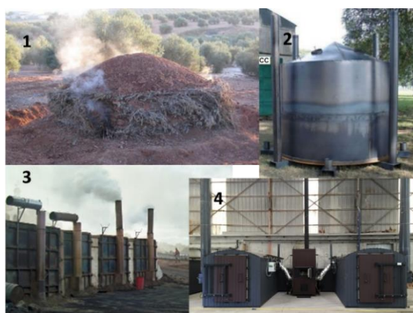
Figure 1: Charcoal production technologies as investigated in this paper: (1) mould earth kiln; (2) metal ring kiln; (3) Missouri type kiln; (4) modern metal kiln with gas recycling
