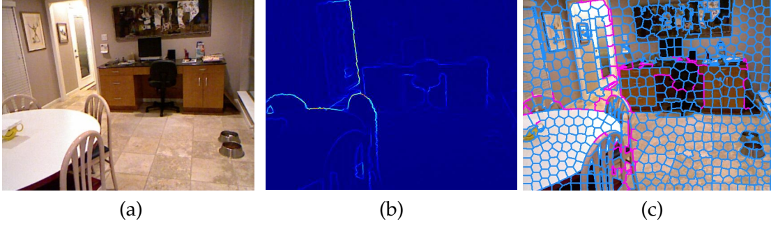
Figure 3.4: An example of boundary occlusion map: (a) Image; (b) depth gradients, where color indicates gradient (red is large, blue is small).; and (c) ground truth boundary occlusion map. The boundary occlusion is labelled in purple.
