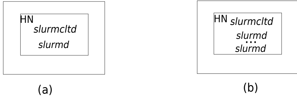
Figure 3.2: Cluster emulation using Slurm Front End and Multiple slurmds features. (a) A single slurmctld and single slurmd can run in the Head Node (HN), or in a desktop, if Slurm is compiled with the Front End option. In this case, the emulated nodes will be set up in the Slurm configuration file but all job management will be accomplished by the single slurmd . (b) Additionally to the Front End option we can also run multiples slurmds in a single computing node with the Multiple Slurmd option. As in (a) the emulated nodes will be also set up in the configuration file, but the management of all the jobs will be shared between the several slurmds .
