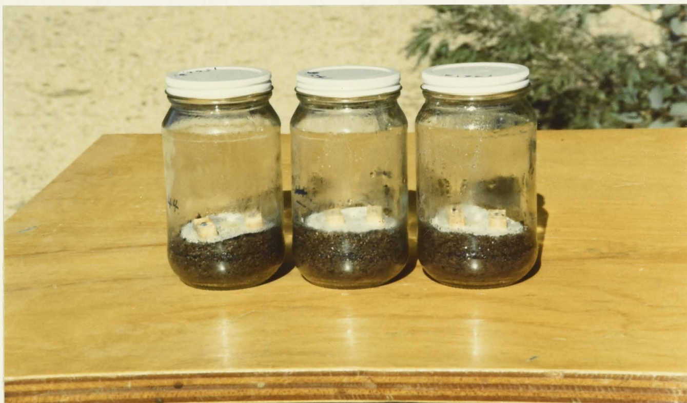
Plate 2-4: Wood-block/soil-jar decay assembly containing moist sandy-loam top soil (nutrient-rich base) covered with a filter paper feeder strip which is overgrown by vigorous mycelial mat of the test fungus. The wood blocks are decayed by white-rot organisms
