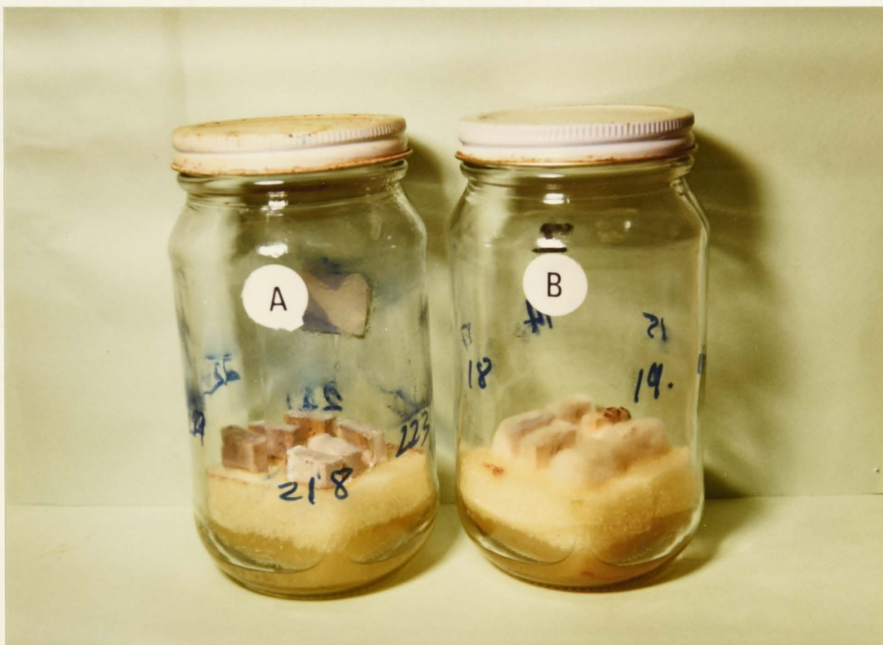
Plate 2-5: Wood-block/foam-jar decay assembly with polyurethane foam (nutrient-depleted base) soaked in sterile deionized water. The wood blocks are decayed by a white-rot (A) and a brown-rot (B) organism
