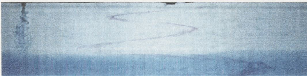
Figure 4.8. The shear layer structure had already developed throughout the tank by the time the dyed outflow from a restarted plume in a previously established density gradient had been advected to \zeta = 0.65 .
