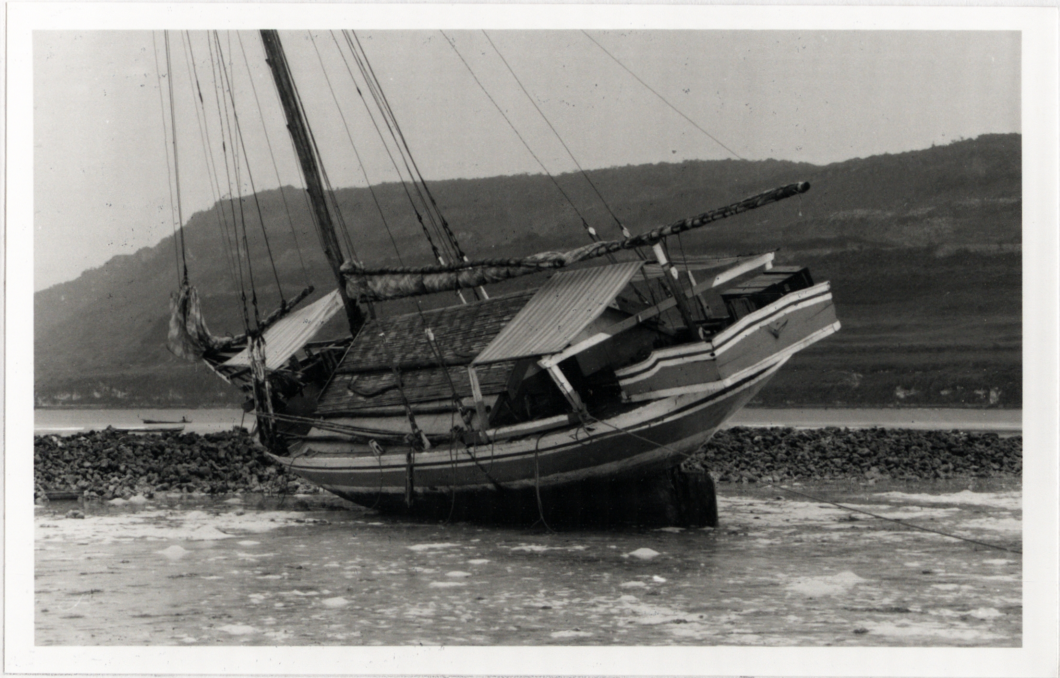
Photos 2 & 3. Perahu lambo careened at low tide for maintenance work.
