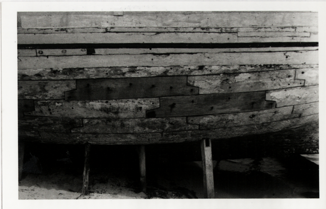
Photo 5. The hull of a perahu lambo with the lime caulking removed to show the plank design. Note the parapalea joint.
