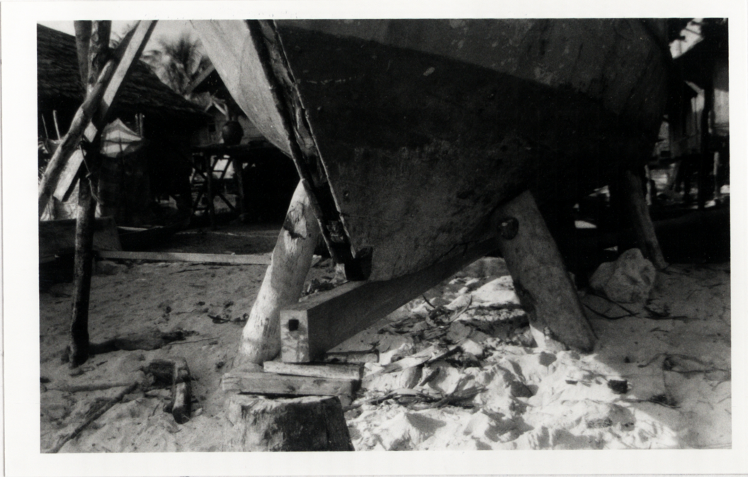
Photo 4. The new keel of a perahu under repair, showing the mortice joint. The keel comprises a single length of timber instead of three sections since this is an engine-powered perahu. The three-section keel is considered to be too weak to bear the weight and vibration of an engine. Note also that the new keel is longer than the old keel; the length of the boat will be increased slightly.
