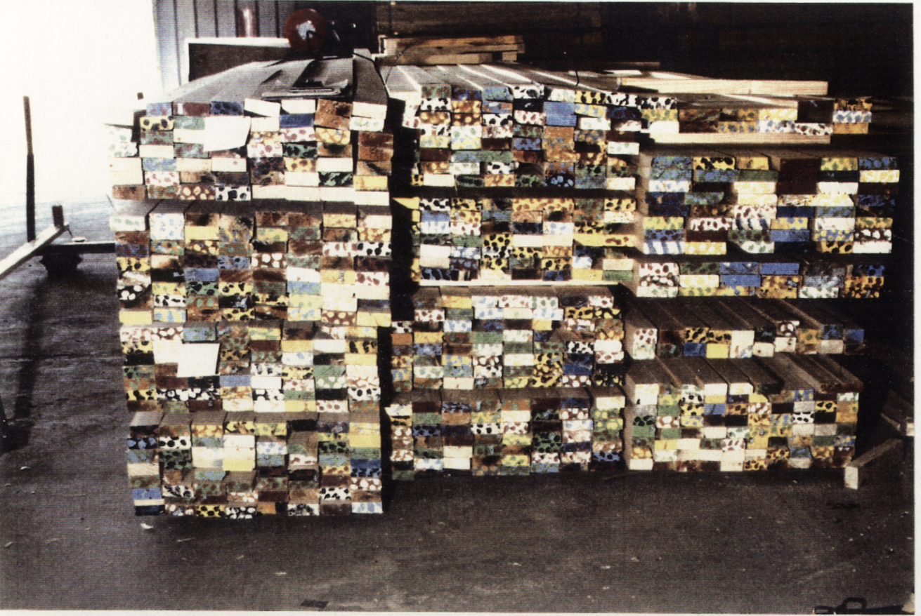
Plate 6.2 Stack of framing timber , illustrating machine stress grades
