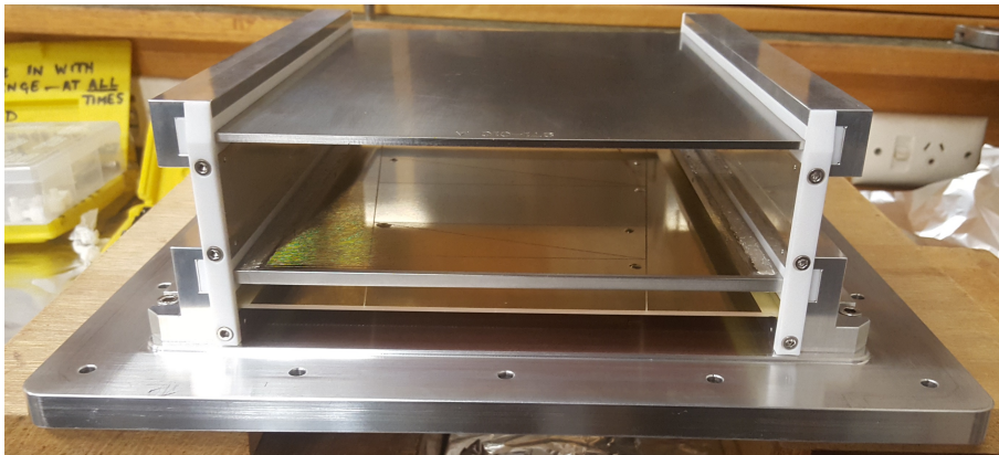
(b) The electrode stack with its slide-in utility. Note that the soldering bumps on the anode were later redone to lay flush with the anode.
