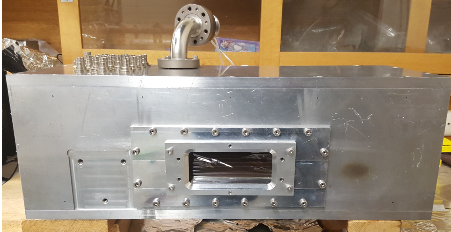
(a) Aluminium housing for the current detector.
