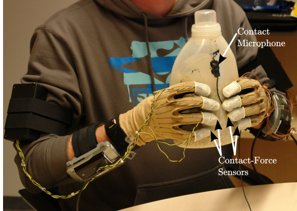
Figure 1: Experimental setup: a human demonstrator wearing contact sensors performs manipulation operations with a plastic bottle equipped with a structure-borne microphone. The CyberGlove trajectories also recorded in this scenario are not evaluated in this work.
