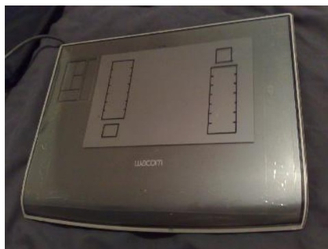
Figure 8: The interface for the Connect Four game on the graphics tablet. The interface is inverted, allowing players to sit opposite each other as shown in figure 7.
