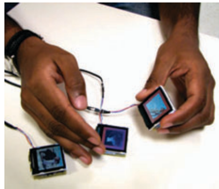
(d) Prototype of Siftables (graphic reproduced from [MKM07] by courtesy the author)
