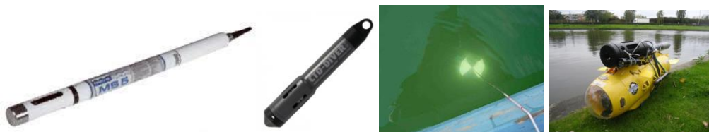
Figure 3: Measurements equipment from left to right: Hydrolab MS5 probe, CTD diver, Secchi Disk and Thunder Tiger Neptune SB-1 underwater drone.
