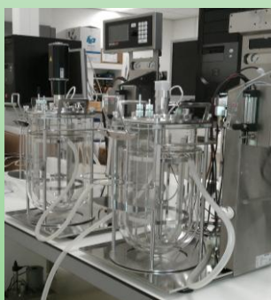
Figure 4: Two Infors 13 liter Lab-scale Bioreactors:
