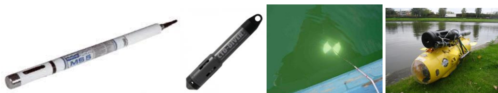
Figure 3: Measurements equipment from left to right: Hydrolab MS5 probe, CTD diver, Secchi Disk and Thunder Tiger Neptune SB-1 underwater drone.
