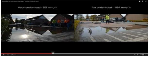
**Figure 6** visualisation by time-lapse camera showed the infiltration capacity before and after maintenance of permeable pavement at the same time on video (<u>http://www.climatescan.nl/page?details=60</u>). (Tipping, 2015)
