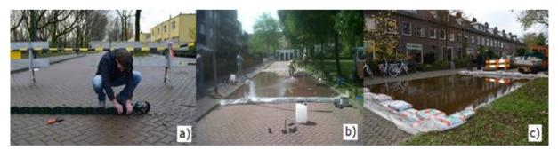
**Figure 3** Various Dam Variations Used at the Different Test Locations (a) Impermeable barriers; (b) Plastic wrapped soil core; (c) Soil-filled plastic bags.
