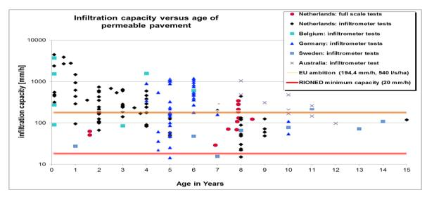
Figure 5 International permeable pavement infiltration capacity research results [Boogaard, 2015]
