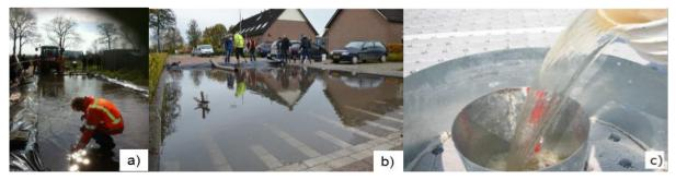
Figure 2. Full scale testing in the Netherlands (a) Impermeable barriers; (b) Plastic wrapped soil core; (c) DRIT testing
