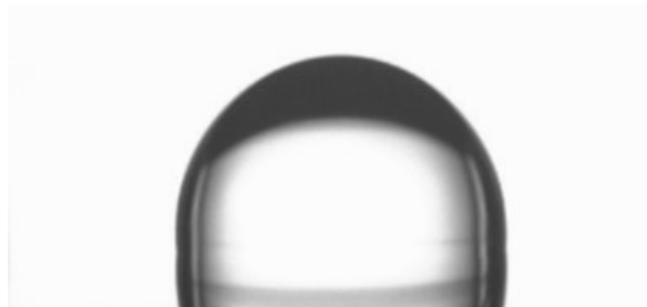
Fig. 3.15: Photograph of droplets placed on the heated after surface preparation.
