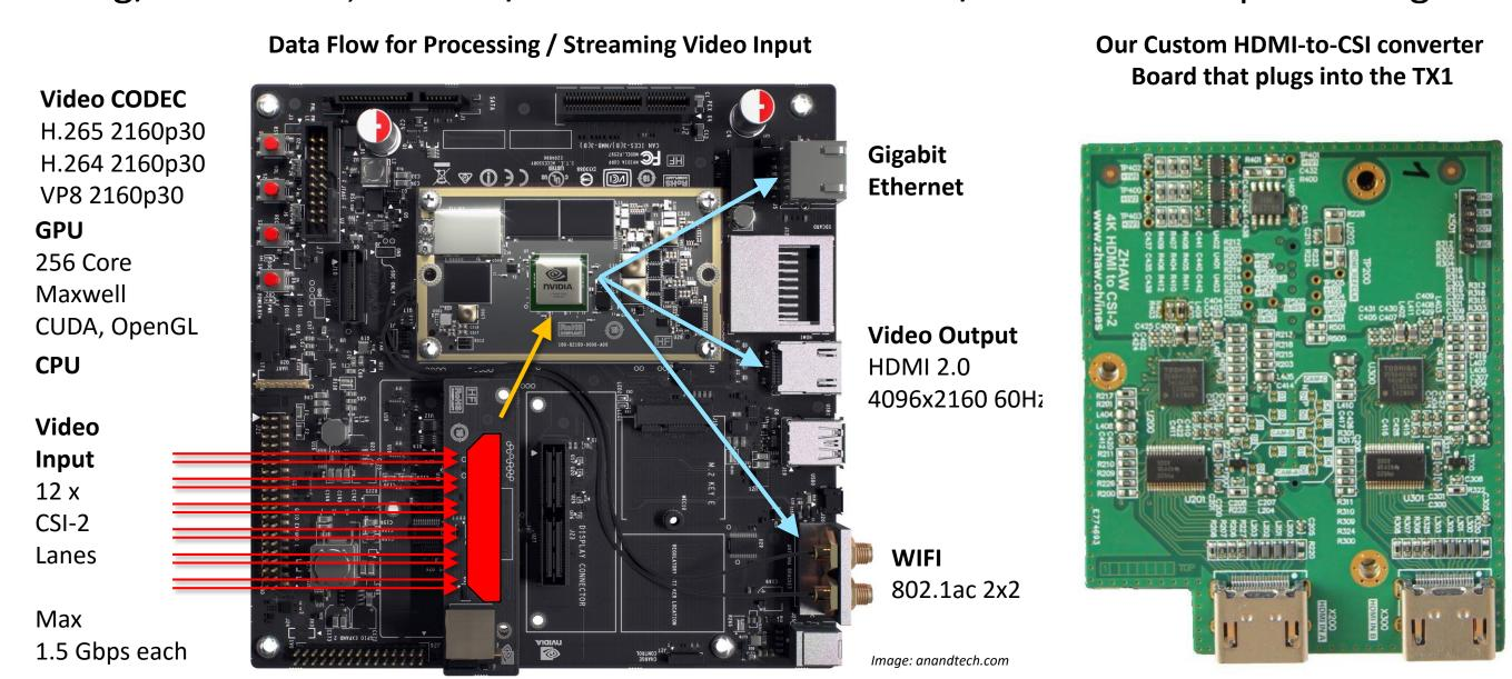
For our use case we had to capture 4K and 1080p simultaneously from two HDMI sources. The Toshiba TC358840 is a HDMI-to-CSI bridge IC, which can convert 4K HDMI inputs to 8 lanes CSI-2. Officially MIPI CSI-2 only supports up to 4 lanes in parallel. Therefore it was necessary to expand the drivers and implement a 4+4 lane «dual link» configuration.
