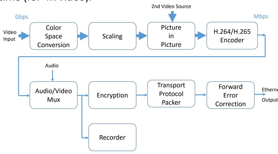
The TX1 provides 12 MIPI CSI-2 lanes which are capable of processing up to 1.5 Gbps of video input data per lane. The TX1 provides powerful hardware-accelerated video scaling/conversion, a H.264/265 CODEC and the CPU/GPU for video processing.
