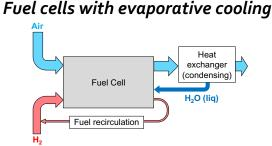
Cost reduction: novel evaporatively cooled fuel cell design
