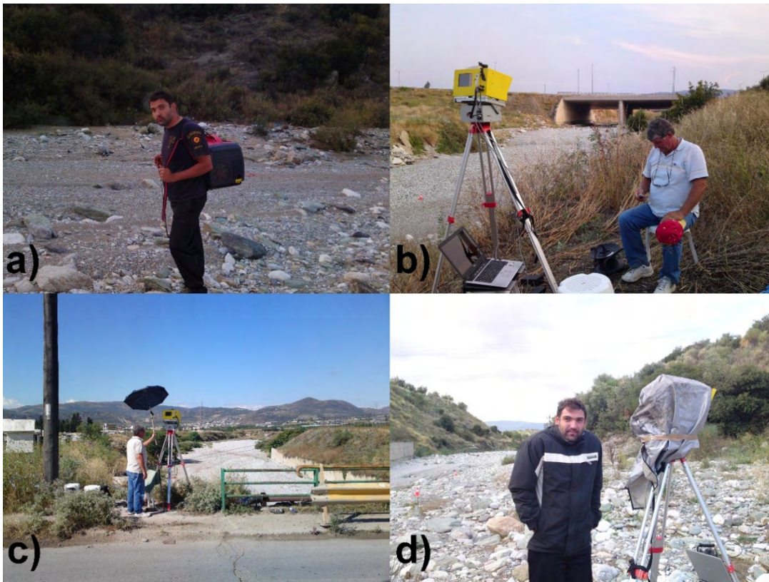
Figure 3.3. Difficulties encountered during the scanning procedure: a) Carrying heavy equipment; b) Settle down the equipment and wait for the scanning procedure; c) Protect the equipment from high temperatures; d) Protect the equipment from low temperatures.
