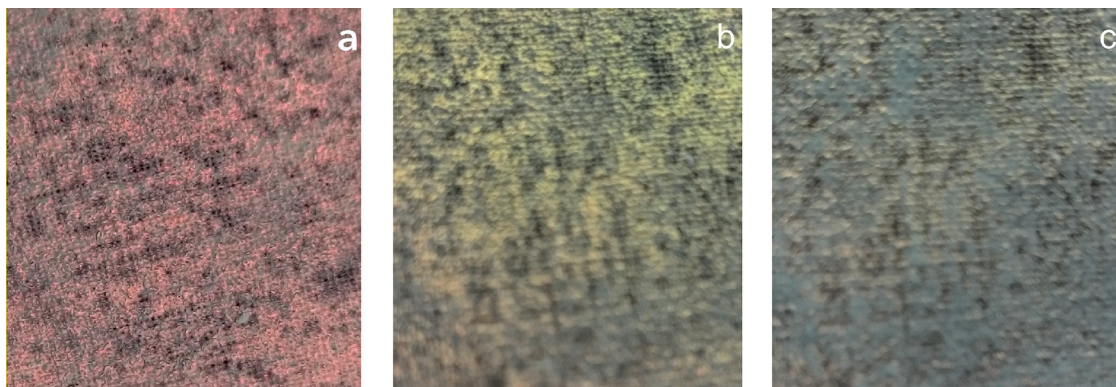
Fig. 7. Photographs of the crosslinked nanophotonics-coated cationized cotton sample at different angles: a) 0°, b) 45° and c) 90°.
