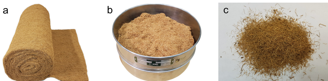
Fig. 1. (a) As-received reel of coconut fibers (CFs); (b) Ground CFs; (c) Sieved CFs.
