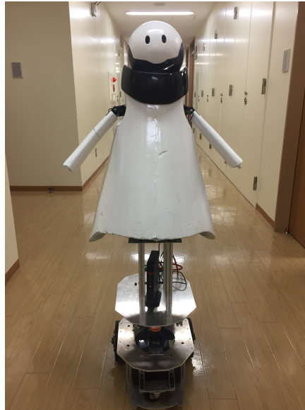
FIGURE 4.1: Gemini: the new designed humanoid walking companion
