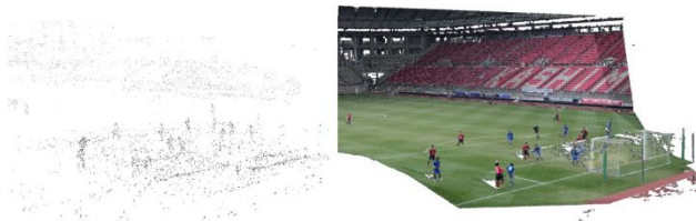
Figure 5: Left: point clouds restored by SfM; Right: point clouds restored by stereo method.
