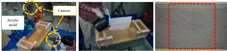
Figure 1. Visualization simulation using water glass.
