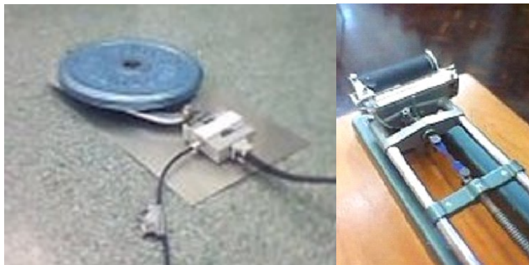
Figure 8: Apparatus used to determine both friction co-efficient and flow stress of closure material respectively.
