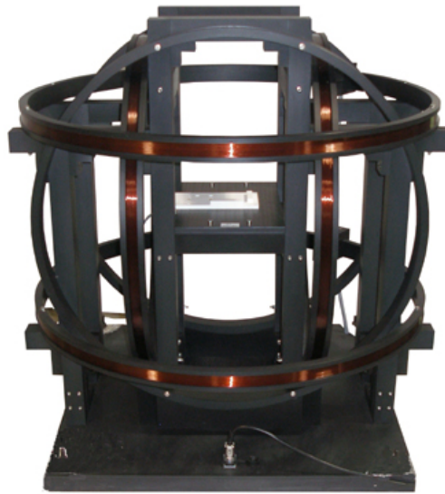
Figure 5.1 : A 3 axis, circular Helmholtz coil system [13].
