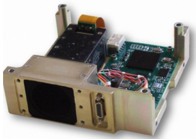
Figure 2.5 : A Star tracker as a subsystem with dimensions of 10cmx10cmx3cm [7].
