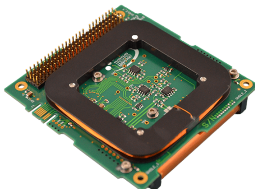
Figure 2.6 : A magnetorquer coil on upper side and a rod on lower side [8].
