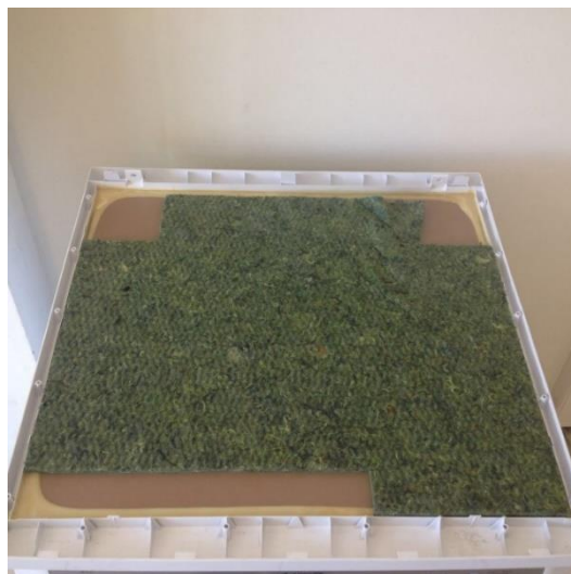
Figure 5.11 : Felt applied into the washing machine body.
