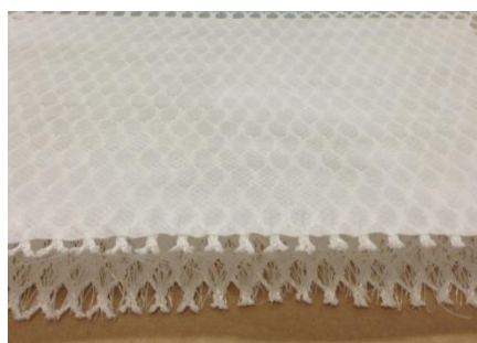
Figure 5.9 : Nanofibrous membrane with spacer knitting substrate.
