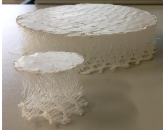
Figure 5.20 : Combined structures with knitted spacer substrates.
