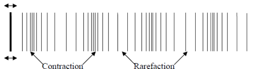
Figure 3.1 : Radiation of sound waves from an oscillating body [73].
