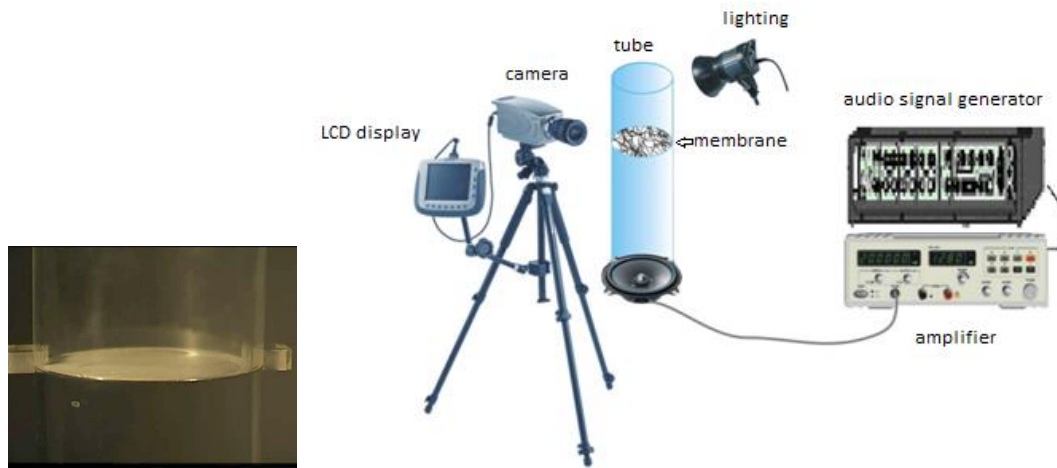
Figure 5.15 : Scheme of the measuring system with the detail of real membrane setting inside the tube.
