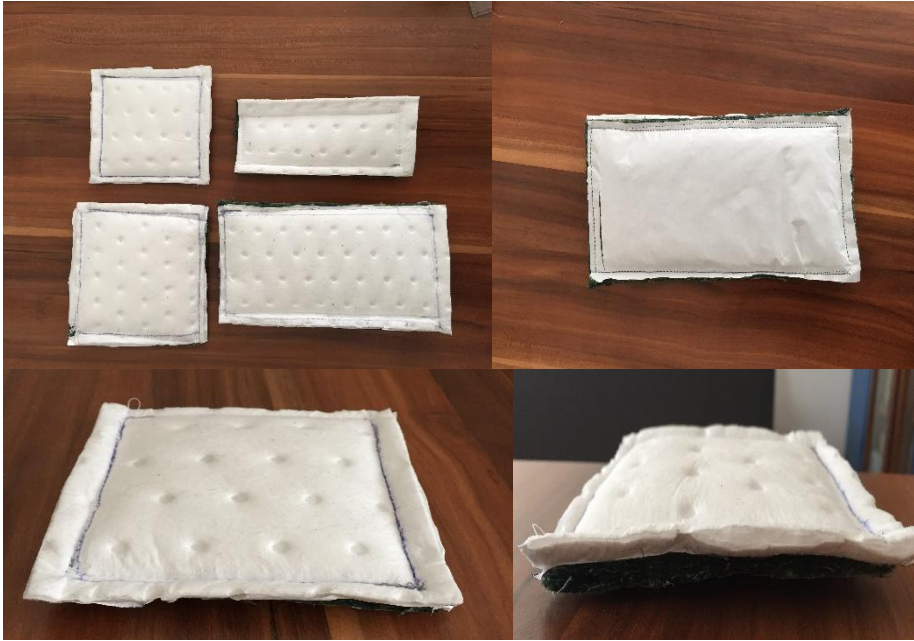
Figure 5.10 : Combined structures comprising wool felt, nano membrane and the covering layer.
