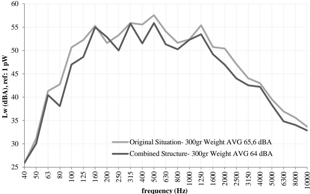
Figure 6.93 : Comparison of Sound Power Level Measurements in the case of 300 gr weight in washing machine.
