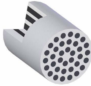
Figure 2.5 : Typical bicomponent islands-in-the-sea fiber [12].
