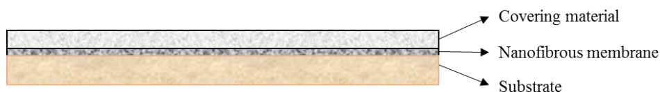
Figure 5.5 : The combined structure.
