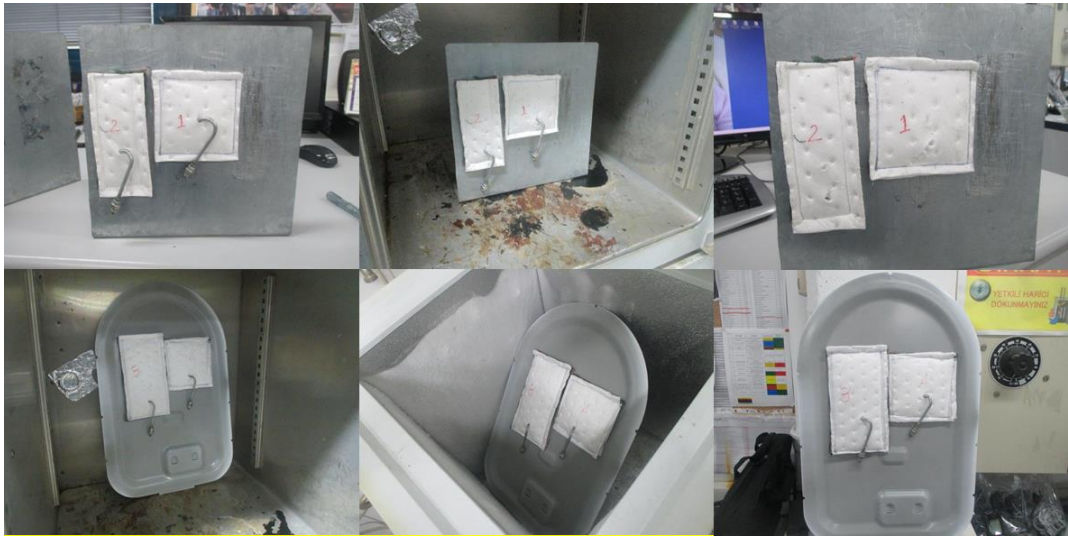
Figure 6.94 : The combined structure that passed the adherence tests.
