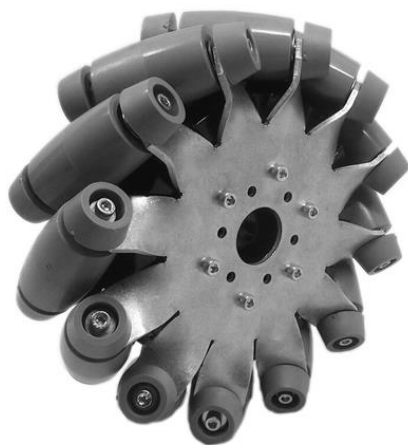
Figure 3.2: Mecanum wheel with 12 rollers
