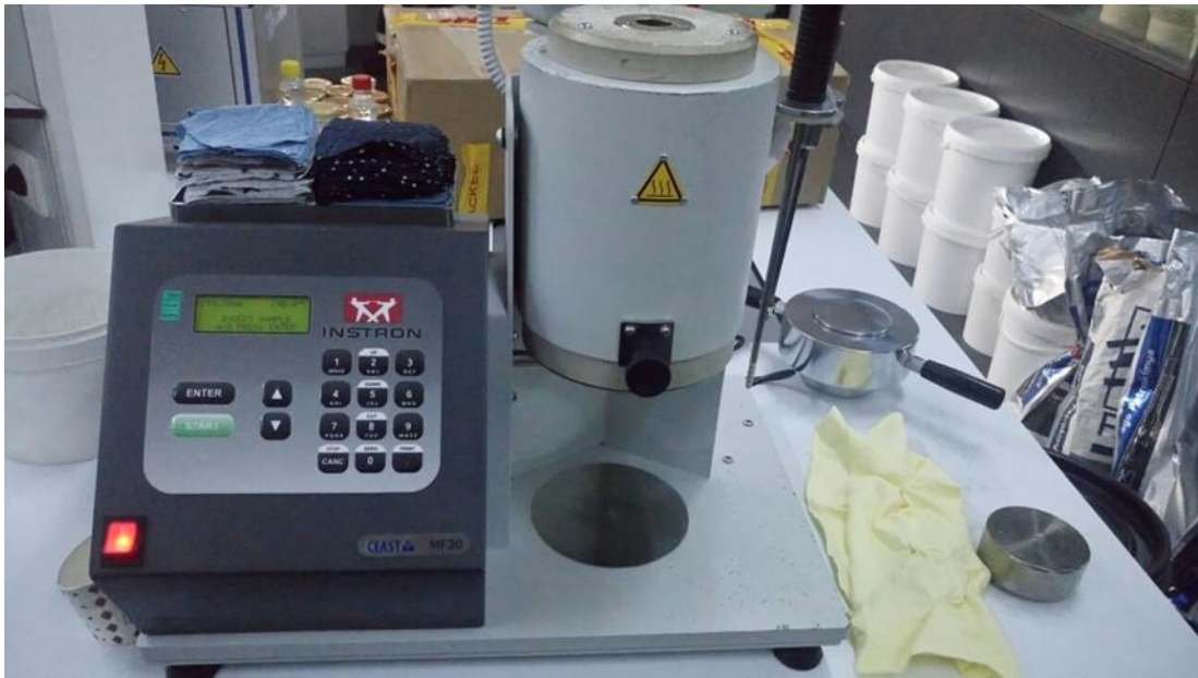
Figure 3.10 : Melt Flow index test device
