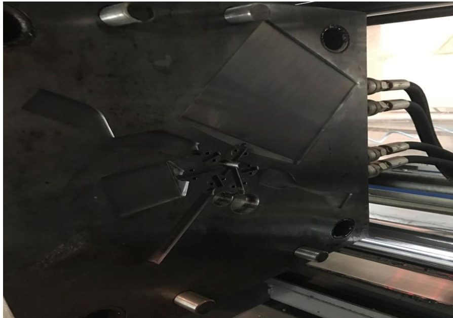
Figure 3.3 : The mold shape in injection molding machine
