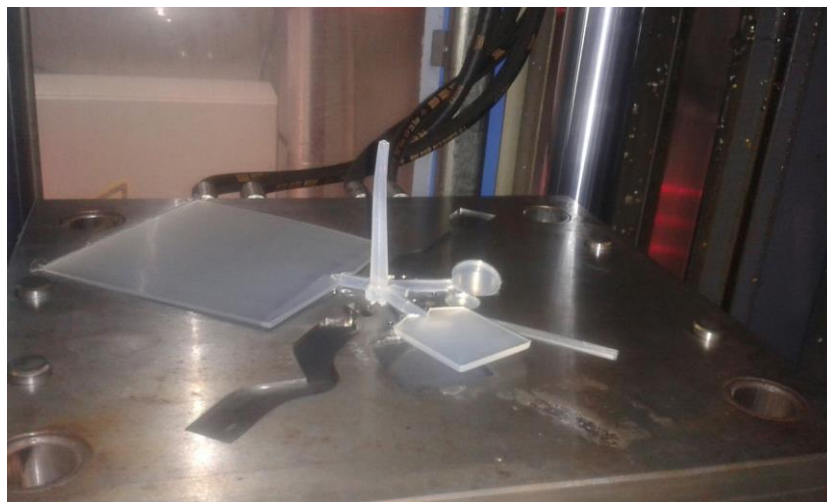
Figure 3.4 : The test specimens after the molding
