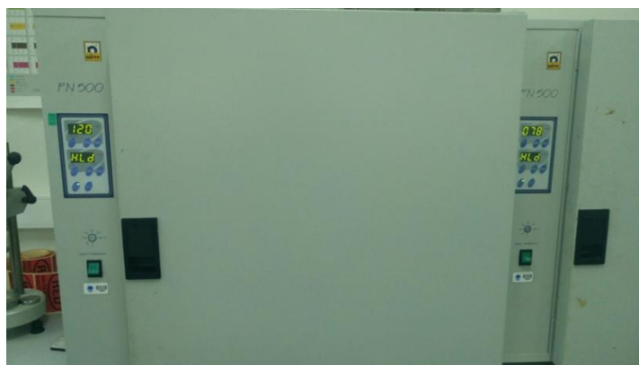
Figure 3.14 : Nuve- FN 500 for drying the pellets.
