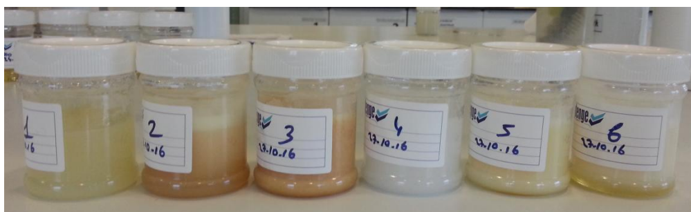
Figure 3.12 : Silicone emulsions used in experiment 6.
