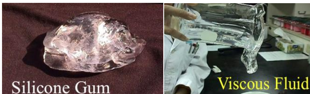
Figure 2.12 : Gummy silicone gel vs. viscous silicone fluid.
