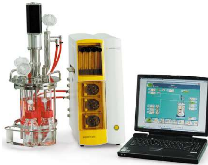
Figure 2.3: The Biostat A Plus (5L) bioreactor and computer based control program.
