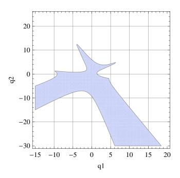
**Figure 5.5** :  $q_1 - q_2$  region that make the closed loop uncertain system stable.
