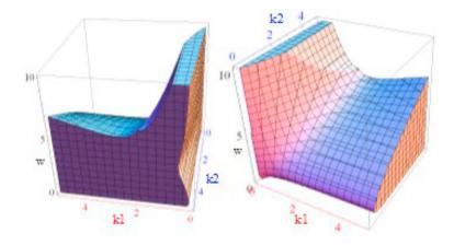
Figure 5.2 :  $k_{p_1} - k_{p_2}$  region that makes the closed loop parameter uncertain system diagonal dominant at  $10 \ge \omega \ge 0$ .
