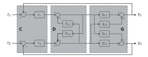
Figure 2.3 : Inverted decoupler block diagram.
