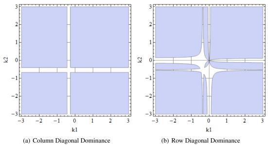
Figure 3.2 : Controller parameter regions for diagonal dominance at  $\omega = 0$ .
