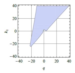
**Figure 5.4** :  $k_1 - q$  region that make the closed loop uncertain system stable.
