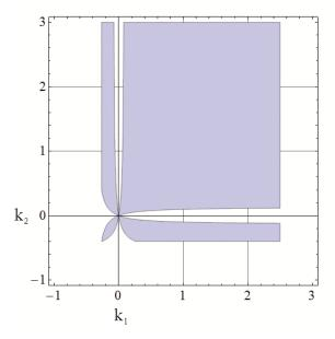
Figure 4.12 : Case study III: Parameter regions that achieve both diagonal dominance conditions at  $\omega = 0$  rad/s and stability criteria.
