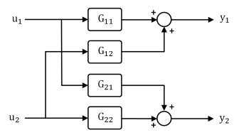
Figure 2.1 : Process interaction in a TITO system.
