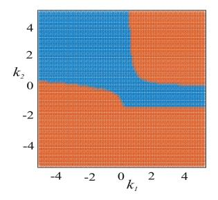
Figure 5.8 : Derived  $k_1 - k_2$  region that make the closed loop uncertain system stable by griding uncertain parameters.
