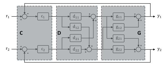
Figure 2.2 : Conventional decoupler block diagram.
