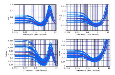
Figure 5.3 : Diagonal dominance ratio plots for parametric uncertain system for  $10 \ge \omega \ge 0$ .
