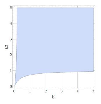
Figure 5.1 :  $k_{p_1} - k_{p_2}$  region that makes the closed loop parameter uncertain system diagonal dominant at  $\omega = 0$ .
