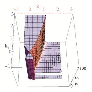
**Figure 4.13** : Case study III: Parameter regions that achieve both diagonal dominance conditions for 100  $rad/s \ge \omega \ge 0$  rad/s and stability criteria.
