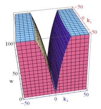
**Figure 3.11** :  $k_{p_1} - k_{p_2}$  regions that achieve CDD and RDD for  $100 \ge \omega \ge 0$  $(\mu_{c_1}, \mu_{r_1}, \mu_{c_2}, \mu_{r_2} = 2).$
