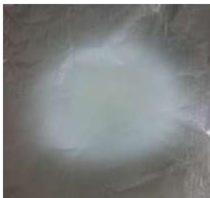
Figure 3.1 Nanofiber on an aluminum foil from chitosan and PVA dissolved in acetic acid.
