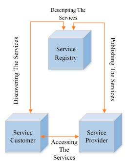
Figure 3. Service-Oriented Architecture (SOA) [15].
