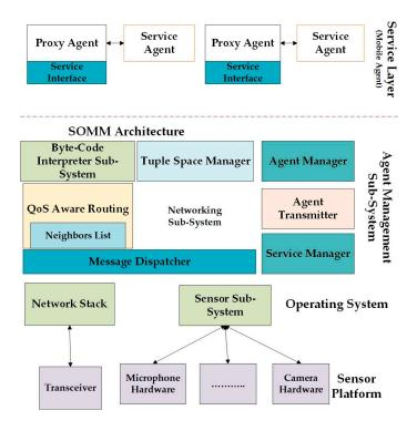
Figure 7. SOMM Architecture in the Server Node [51].
