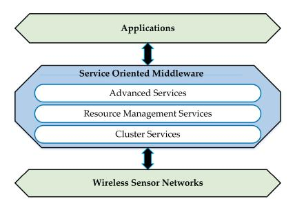
Figure 2. The SOM Architecture Layers for WSNs [4].
