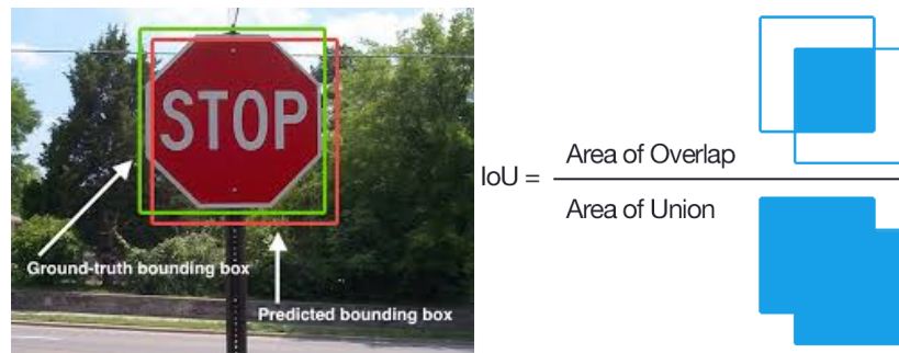
Figure 23. Intersection over Union (IoU) [25]
