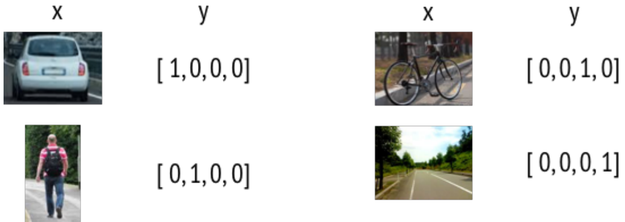
Figure 10. Data labelling for CNN classification
