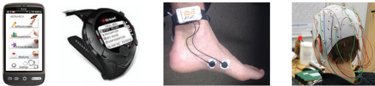
Figure 1.1: The MONARCA solution's 4 components. From the left the Smartphone, the wrist worn activity monitor, the “sock integrated” physiological sensor, and the stationary EEG system.
