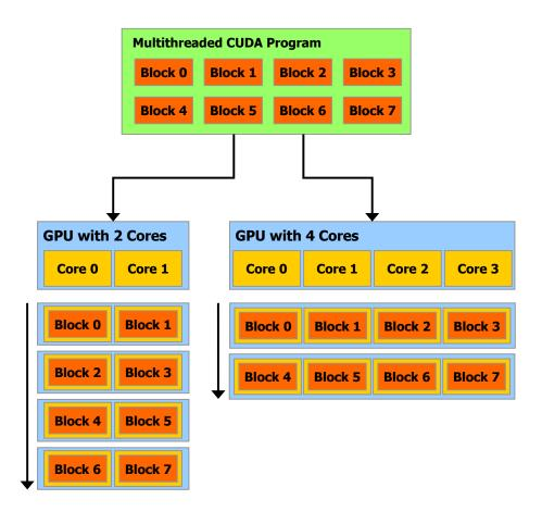
Figure 4.7: Transparent thread scalability, taken from [NVI10]
