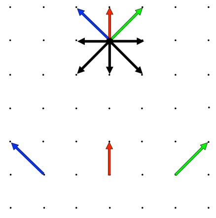
Figure 3.5: Stream step for a periodic boundary
