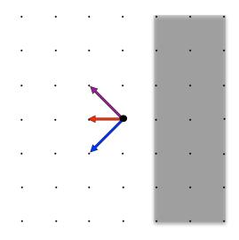
Figure 3.9: Post–Stream step for a bounce–back boundary for a time t + dt
