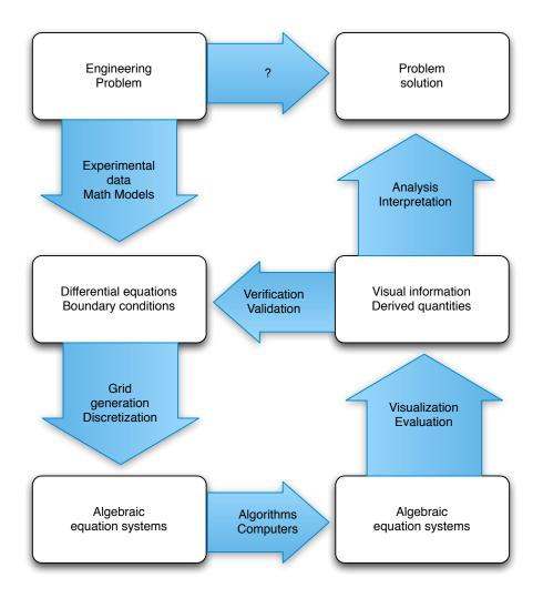
Figure 1.1: Numerical simulation procedure of engineering problems (Schäfer).
