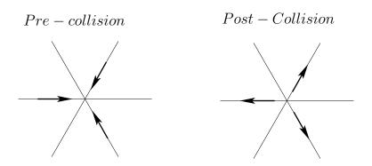
Figure 2.5: FHP three particle head on collision rule
