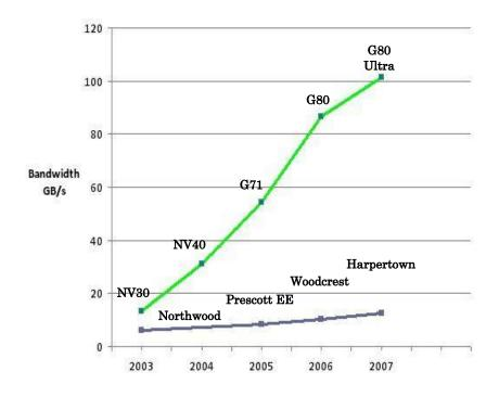
Figure 4.3: Memory bandwidth for the CPU and GPU, taken from [NVI10]
