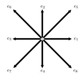
Figure 3.3: Vectors of the D2Q9 lattice.
