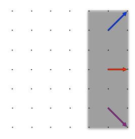
Figure 3.7: Post–Stream step for a bounce–back boundary for a time t
