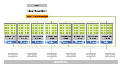
Figure 4.4: Modern GPU architecture, taken from [KmWH10]
