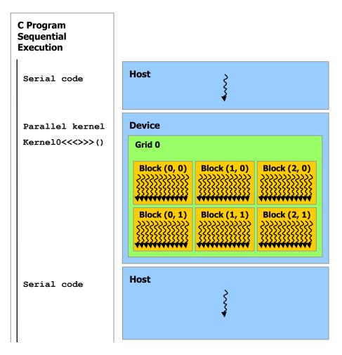
Figure 4.5: Heterogenous programming model, taken from [NVI10]
