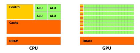
Figure 4.2: Design difference between GPUs and CPUs, taken from [NVI10]
