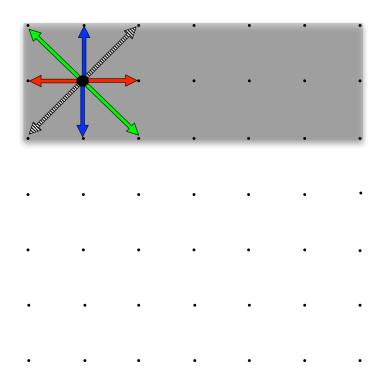
Figure 3.12: Post–Stream boundary node showing bounced direction–specific densities
