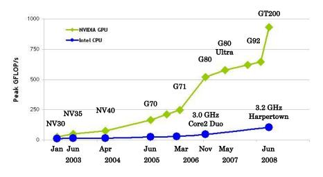
Figure 4.1: Performance gap between GPUs and CPUs, taken from [NVI10]
