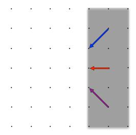
Figure 3.8: Bounce-back of direction-specific densities
