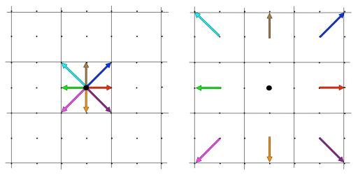
(a) Discrete direction–specific densities (b) Discrete direction–specific densities for for time t time t + dt
