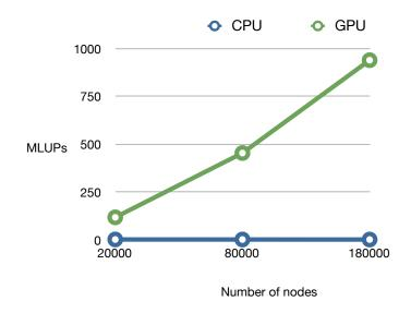
Figure 6.2: Acceleration gained using GPU
