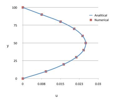
Figure 6.1: Predicted velocity profile of Poiseuille flow
