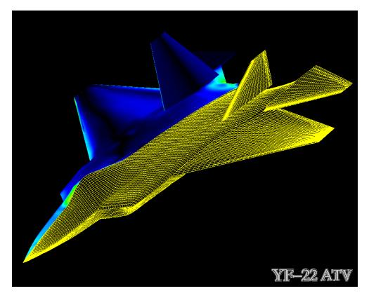
Figure 1.2: Mesh of an F–22 airplane(NASA).
