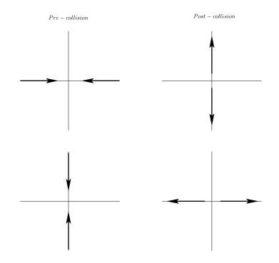
Figure 2.2: HPP collision rules
