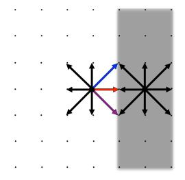
Figure 3.6: Pre–Stream step for a bounce–back boundary for a time t
