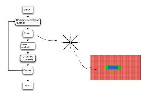
Figure 4.9: LBM runs the same algorithm over each node of grid
