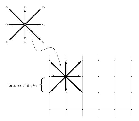
Figure 3.1: LBM cartesian grid and vectors of the D2Q9 lattice.
