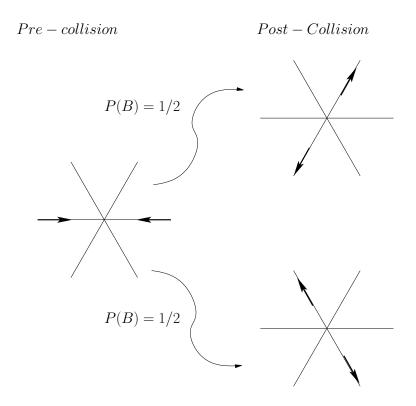
Figure 2.4: FHP collision probability
