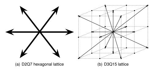
Figure 3.2: Two common lattice schemes for the Lattice Boltzmann Method
