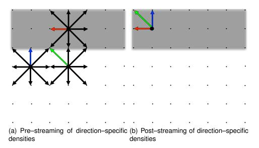
Figure 3.11: Corner node problem of boundary condition
