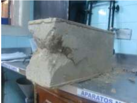
Figure 3. 4. Diagonal crack, typical in low strength blocks.
