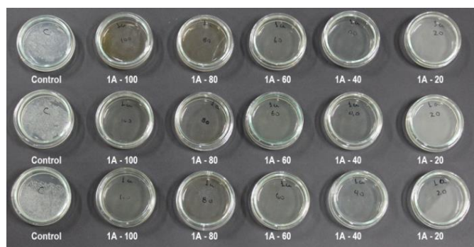
Figure 3: Photographs of the antibacterial test results of AgNPs at 100, 80, 60, 40 and 20% , made by triplicate.
