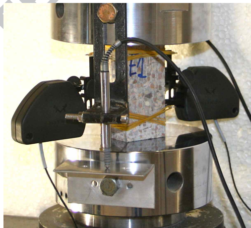
Figure 3: Experimental set-up to measure the elastic modulus.
