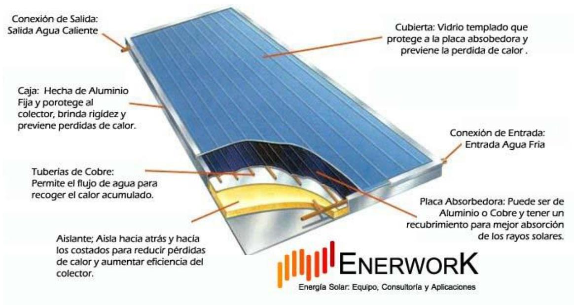
Figura 9. Colector de placa plana ENERWORK [31]
